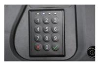
The PIN-code lock can be set with multiple passwords and also supports RFID card activation.
