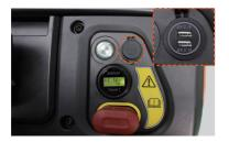
The Multi-functional LCD indicator displays the information about remaining battery power, amount of working hours and fault codes.
