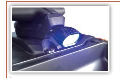
The standard blue light does not only automatically lit while the ruck forwarding but also follows the handle to turn while the truck turns. It greatly improves the safety of the operation.
