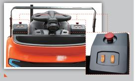
A variety of extension supports are available to The upper adjustable balance wheel can Easier to entry Australian pallet with entry The jog button on both sides of the truck allows the operator to operate truck forward/ backward or lift the fork while walking beside. There is no need for the operator to get in and out of the truck frequently to operate it. That greatly improved the picking efficiency and operation safety by reducing the speed controlled by the jog button.
