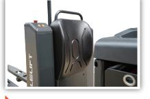
Safety flanks and non-slip surface materials on both sides of Large storage tray can be used for storing the backrest ensure the operator not to be thrown off while the stretch film, art knife, marker pen, or other truck turns at high speed. This design greatly improves the tools. safety of driving. Meanwhile, the handle above the backrest provides a grasping point for the operator when get up or down the truck, provides superior comfort for the operator.
